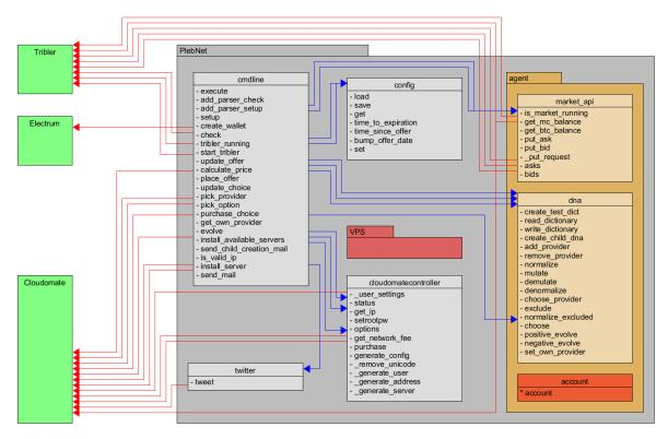
Figure 4.1: Interpackage dependency diagram of the provided code. Blue lines indicate internal dependencies and red lines external. Red files/packages indicate unused code. The amount of arrows between different files indicate the amount of calls made between the files. More lines results in a higher connectivity.
