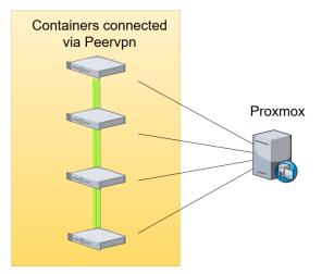
Figure 7.3: Overview of the Proxmox server. Containers are connected with each other through PeerVPN.
