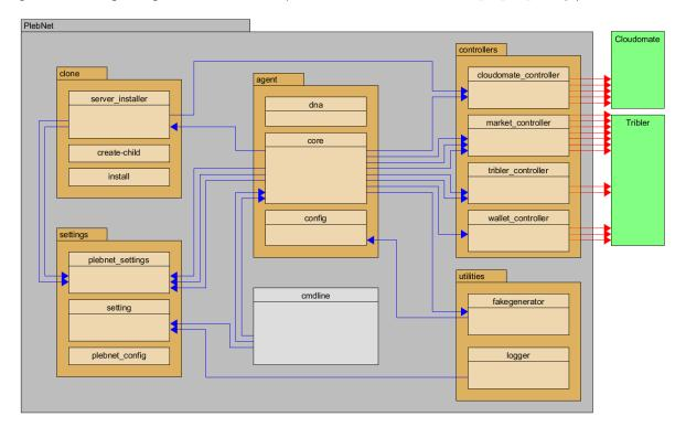
Figure 4.3: Interpackage dependency diagram of the provided code. Blue lines indicate internal dependencies and red lines external. The communication package and the dependencies on the logger are left out for readability as they are not part of the core of PlebNet. The amount of arrows between different files indicate the amount of calls made between the files. More lines results in a higher connectivity.
