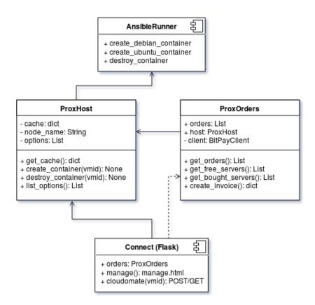
Figure 7.4: A simplified UML diagram of the end-to-end system. The Flask component "Connect" allows Cloudomate or web users to purchase containers. When a purchase is made, ProxOrders creates an invoice which Connect returns as a HTTP response. ProxHost can either create or destroy containers by creating an AnsibleRunner object with the appropriate parameters.
