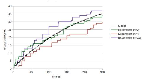
Figure 6.7: Measurements of content discovery: releases discovered after a fresh installation. n: network size (amount of Android devices)
