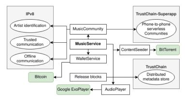
Figure 4.1: Architecture overview, with in green the external software components. MusicService is the central component in our system
