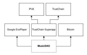
Figure 5.1: The main external components used in MusicDAO
