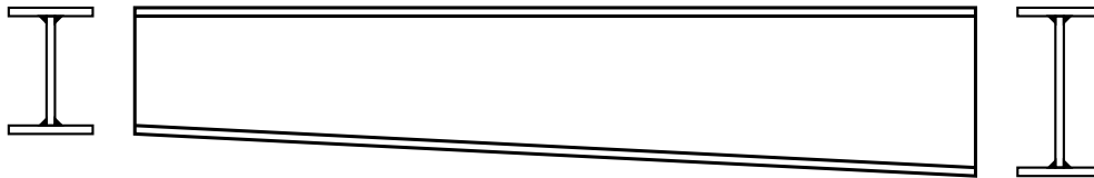
Figure 2.10: Non-prismatic sections by plates welded together
