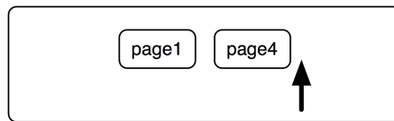
Figure 15-11 From page 1, the user clicks on a link to page 4. The history forgets pages 2 and 3.
