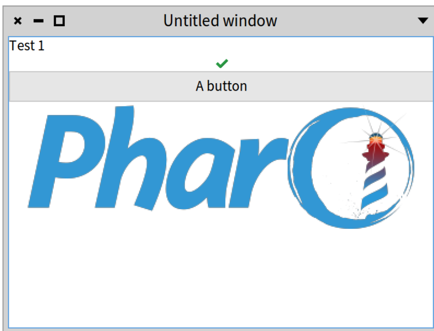
Figure 8-7 A component list with several different presenters: a label, an image, a button, and an image. %width=45&anchor=figCompo
