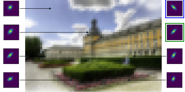
Figure 3: Kernel estimation results of the proposed MANet under consecutive degradation when scale factor is 4. The testing image is “img077” in Urban100 [4]. We blur and downsample the HR image twice with two different kernels (in total, 16\times ), which are shown in the blue and green rectangles. The shown image is the 4\times nearest neighbour interpolation of the final LR image.
