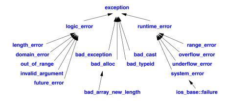
This hierarchy attempts to provide a framework for exceptions beyond the ones defined by the standard library. Logic errors are errors that in principle could be caught either before the program starts executing or by tests of arguments to functions and constructors. Run-time errors are all other errors. The **system\_error** is described in §30.4.3.3.
