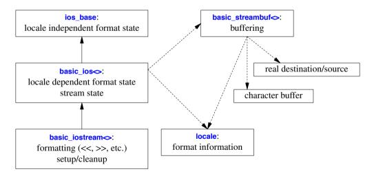
The solid arrows represent "derived from." The dotted arrows represent "pointer to." The classes marked with  $\diamond$  are templates parameterized by a character type and containing a locale.
