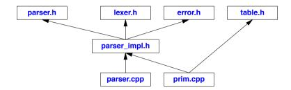
Such elaboration is not appropriate except for larger modules. For realistically sized modules, it is common to **#include** extra files where needed for individual functions. Furthermore, it is not uncommon to have more than one **\_impl.h**, since different subsets of the module's functions need different shared contexts.
