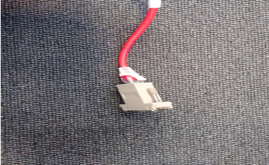
Connecting Network Cable with DB9 Female Connector to RJ45 Female Converter
