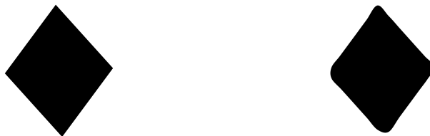
Figure 1.6: A shape with sharp corners (left) and its reconstruction from a low resolution distance field (right).
