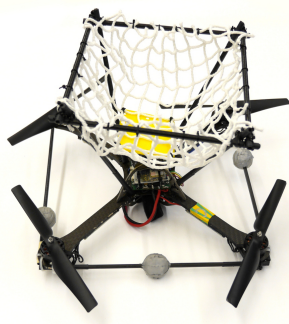
Fig. 6. A quadcopter with attached catching net, as used to demonstrate the algorithm. The centre of the net is mounted above the vehicle's centre of mass in the quadcopter's e_3 direction.
