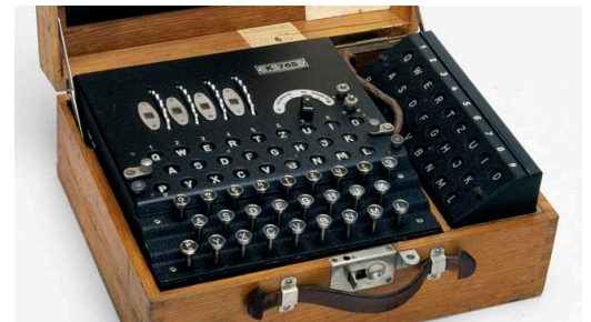
Figure 1.5: In the Enigma mechanical cipher the secret key would be the settings of the rotors and internal wires. As the operator types up their message, the encrypted version appeared in the display area above, and the internal state of the cipher was updated (and so typing the same letter twice would generally result in two different letters output). Decrypting follows the same process: if the sender and receiver are using the same key then typing the ciphertext would result in the plaintext appearing in the display.
