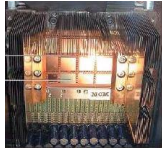
z9 MRU cooling with aircooled backup mode
