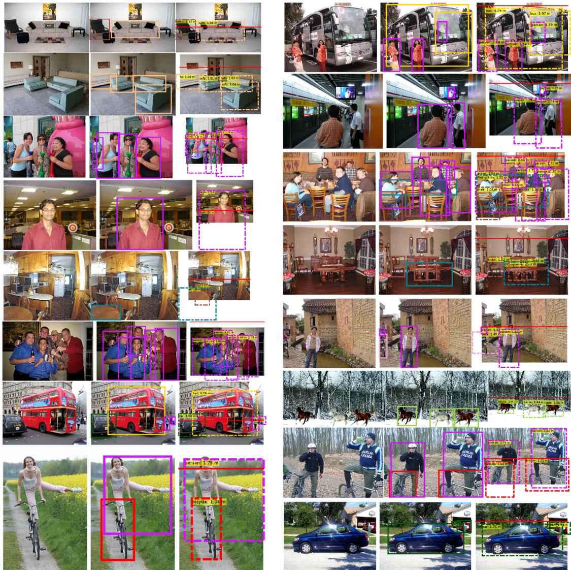
Figure 3.8: Amodal bounding box prediction and size estimation results on images in PASCAL VOC. The solid rectangles represent the visible bounding boxes and the dotted lines are the predicted amodal bounding boxes with heights in meters. The horizontal red line denotes the estimated horizon position for the image.
