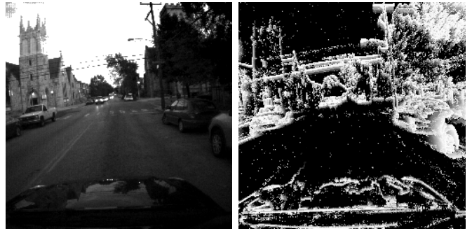
Fig. 3: Example of a timestamp image. Left: Grayscale output. Right: Timestamp image, where each pixel represents the timestamp of the most recent event. Brighter is more recent.
