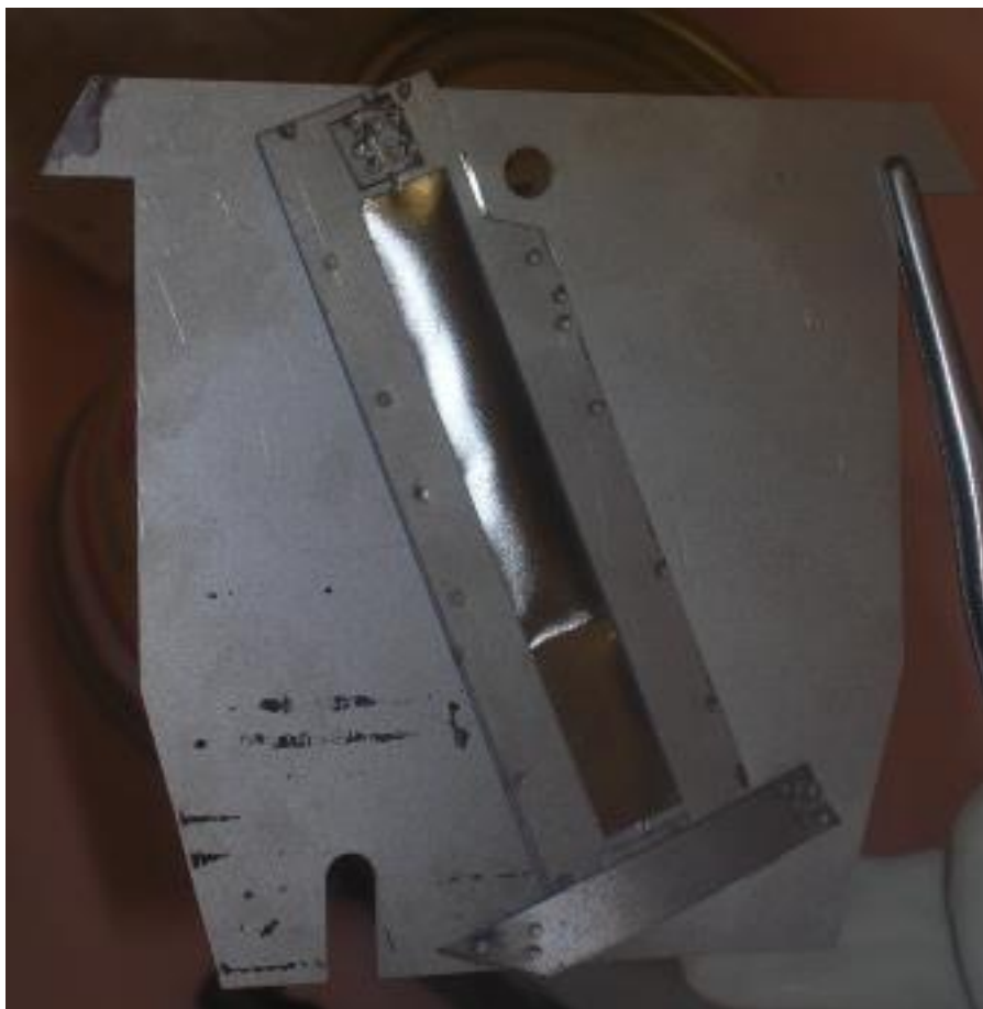
Figure 16. Example of a LOHENGRIN fission target already mounted on the Ti target holder and covered with a thin Ni foil.
