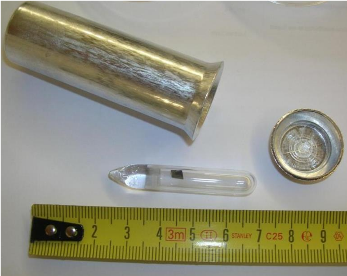
Figure 17. Example of a small metal foil target enclosed in a quartz ampoule to be enclosed into an aluminium capsule for irradiation at ILL.
