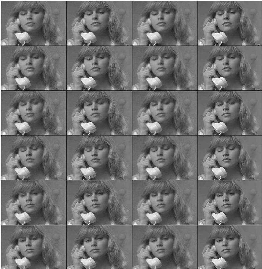
FIGURE 4.4: Results for the 3rd, 8th, 13th, 18th, 23rd, and the 28th frames from the “Suzie” sequence. From left to right: pixel-replicated low resolution image; original image (ground truth); Lanczos interpolation; result of the proposed algorithm.
