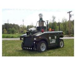
Mobile Detection Assessment Response System - Exterior (MDARS-E) Autonomously conducts surveillance activities checking for intruders, conducts lock interrogations, and assesses the status of facility barriers, such as the doors of storage bunkers.
