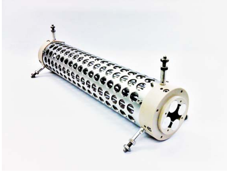
Figure 3.13: Photograph of the quadrupole mass-spectrometer (QMS) required for ion-beam purification. The QMS was developed following design values given in Ref. [194]. The production of a mass-purified ^{229}\text{Th} ion beam is a prerequisite for the unambiguous identification of the isomeric decay. Otherwise, short-lived decay products of the ^{233}\text{U} and ^{232}\text{U} decay chains could not be excluded as signal origin.
