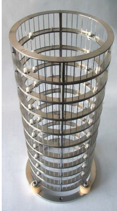
Figure 3.9: Photograph of the DC cage built for the extraction of high-energy nuclear-fusion reaction products. In our experiments, only the last DC-cage electrode was used to provide an electric offset for the ^{233}\text{U} source.
