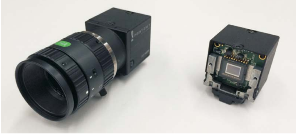
Figure 3.30: Photograph of the CCD camera (Point Grey, FL2-14S3M-C) combined with a zoom lens (Computar M2514MP2, 25 mm, C-mount) used for read-out of the MCP detection system (left). The right-hand side shows the CCD chip (Sony, ICX267 CCD) of an open camera (Photograph from Ref. [217]).
