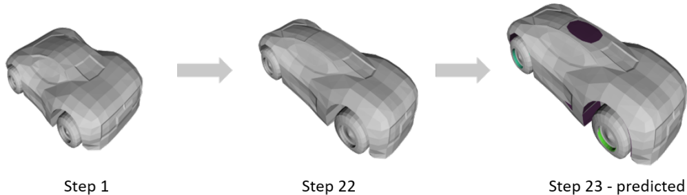
Fig. 6: Design changes predicted by the LSTM model for one sample of design changes: deformed car shape at time-step 1 (left) and time-step 22 (middle) of a representative window. Predicted design changes superimposed on the model from time-step 22 (right). The model proposes to move the roof downward (purple area) and to move the interior of the wheel cover backward (green area).
