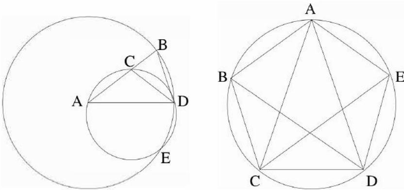
FIGURE 28: *Left*: Euclid's construction of an isosceles triangle with base angles  $4\pi/5$ . *Right*: Euclid's construction of a regular pentagon. Make ACD similar to triangle ABD in the left-hand Figure and proceed from there.
