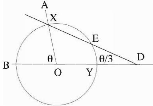
FIGURE 11: Trisecting an angle with a marked ruler.
