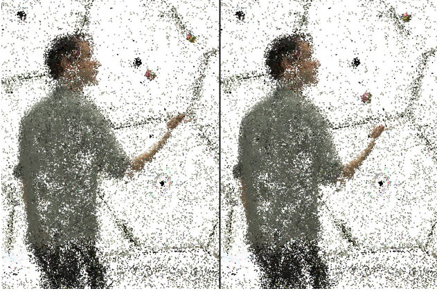
Figure 2. Gaussian Centers. Point-cloud of colored centers in contiguous timesteps, showing how they model scene geometry and move over time. [Videos]
