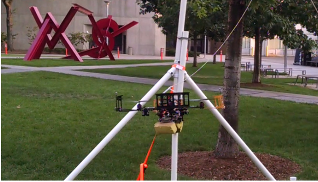
Fig. 5: A series of hover tests were performed in a green space within the MIT campus. The vehicle was autonomously holding position, but tethered to comply with FAA regulations.
