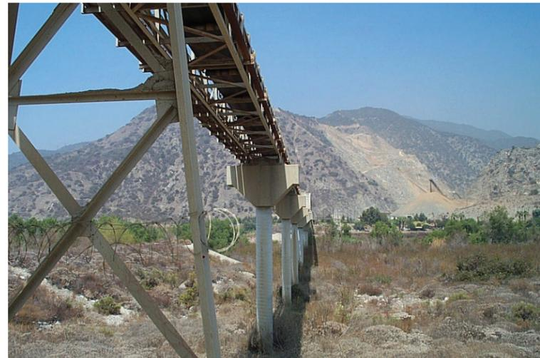
Figure 2-26. Aggregate is carried on a conveyor belt to a processing plant.
