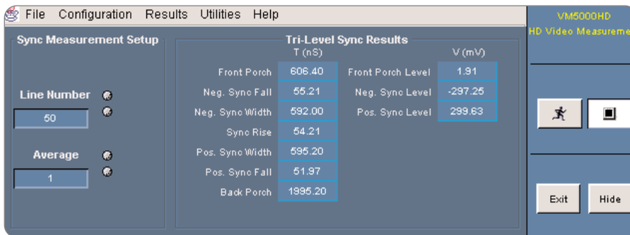
► Figure 16. VM5000HD Sync measurement results.
