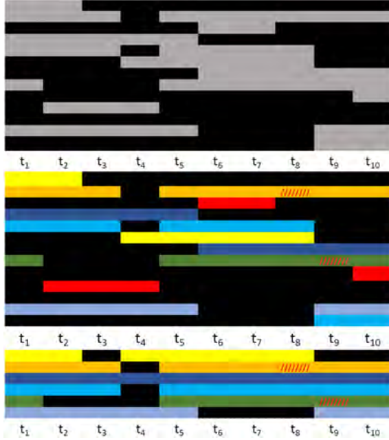
Figure 2: MoCap labeling problem. (top) Raw, unlabeled, MoCap Point Cloud (MPC). Each column represents a timestamp in a mocap sequence and each cell is a 3D point or a short tracklet (shown as a gray row). (middle) shows the MPC after labeling. Colors correspond to different labels in the marker layout. Red corresponds to ghost points (outliers). The red oblique lines show ghost points wrongly tracked as actual markers by the mocap system. (bottom) shows the final result, with the tracklets glued together to form full trajectories with only valid markers retained. Note that marker occlusion results in black (missing) sections.
