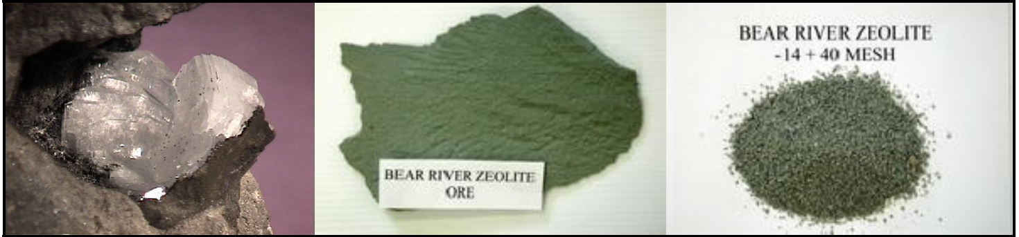
Figure 2: Large crystals of clinoptilolite as cavity filling (amygdule) in basalt (left photo) versus ultra-fine powdered form of clinoptilolite from widespread tuffaceous lacustrine deposits in the western USA [middle and right photos showing clinoptilolite deposits from the Bear River Zeolite (BRZ) mine in Preston, Idaho, the location of the sample for the present study]. Unlike the museum quality hydrothermal (amygdaloidal) form, the sedimentary (diagenetic) form has commercial and industrial importance and pozzolanic properties in concrete.
