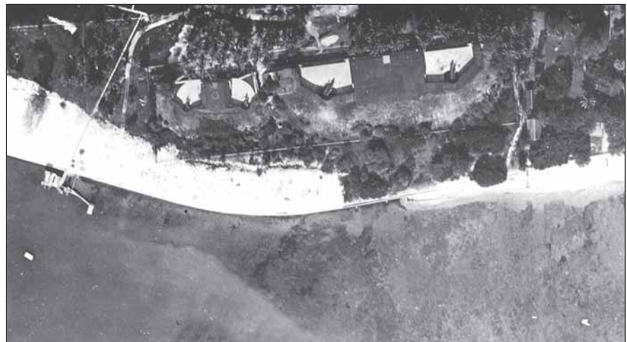
Figure 15. Vertical aerial photo of Fort DeRussy, 21 November 1919; narrow channel dredged in reef connecting to dredged channel in front of new beach. Note diving tower at left. (U.S. Army Museum of Hawaii, USAMH No. 2078.)
