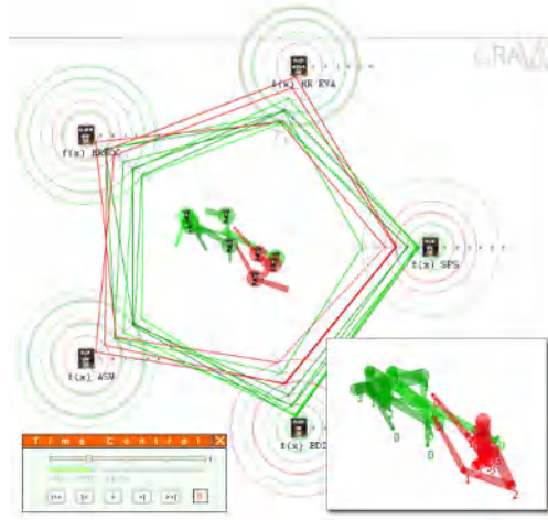
Fig. A.96: Patient icons in the center of the display are positioned relative to the surrounding parameters (in this case items of a questionnaire) following a spring-based model. Individual answers to questionnaire items are shown as concentric rings, and star glyphs show sets of answers as polygonal lines. The user can step through time manually or can use animation, which can be steered via the control panel on the lower left. Furthermore, traces might be displayed to convey information about the evolution of values over time as shown in detail on the lower right. © Courtesy of Klaus Hinum.
