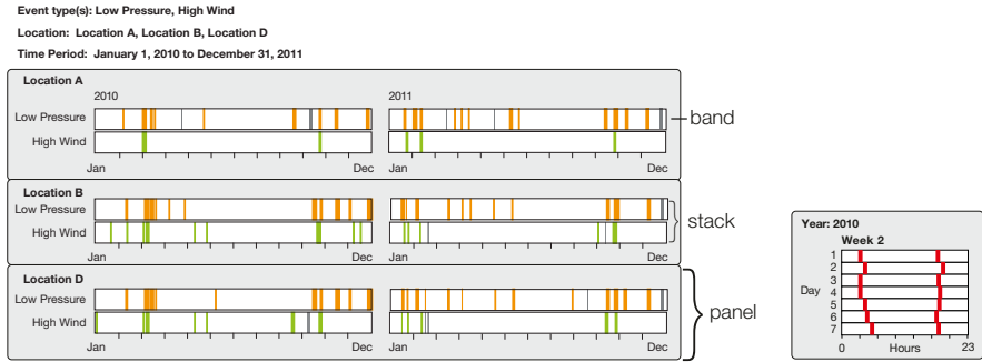
Fig. A.129: Visual exploration of event data via the EventViewer. Spatial, temporal, and thematic dimensions of events can be assigned to configurations of bands, stacks, and panels. Left: low pressure and high wind events are shown along three locations and two years; right: display configuration to reveal temporal patterns along hours of a day. © The authors. Adapted from Beard et al. (2008).
