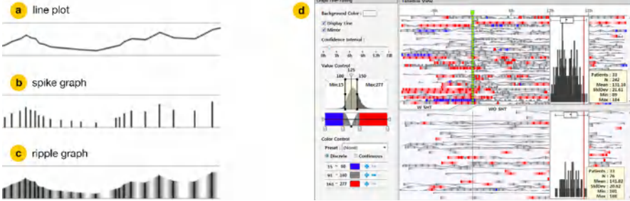
Fig. A.13: Ripple graphs visualize measurement frequency as well as uncertainties of values between measurements. The left part of the figure shows how ripple graphs are constructed: starting from a line plot (a), vertical lines are drawn at the time of measurements resulting in a spike graph (b), finally, color gradients are added to represent uncertainties between measurements (c). On the right, ripple graphs are shown in the context of the Stroscope visualization system. © 2014 IEEE. Reprinted, with permission, from Cho et al. (2014).
