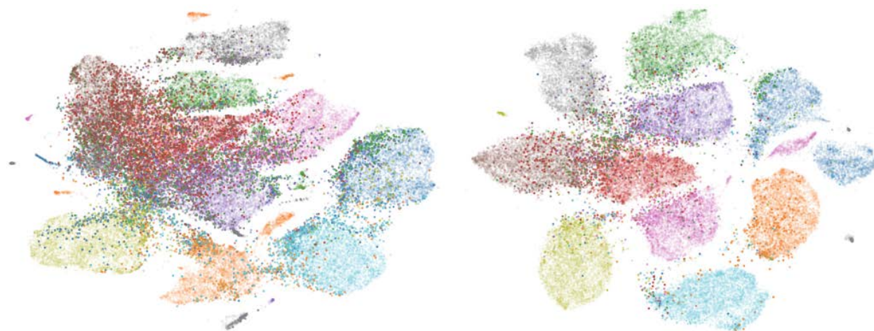
Figure 5.2: LeNet [52] code on the CIFAR-10 [51] training set with importance score represented as transparency of the points. Higher transparency represents lower importance of the data-point to the training process. Left: Codes at Epoch 3, Right: Codes at Epoch 5.
