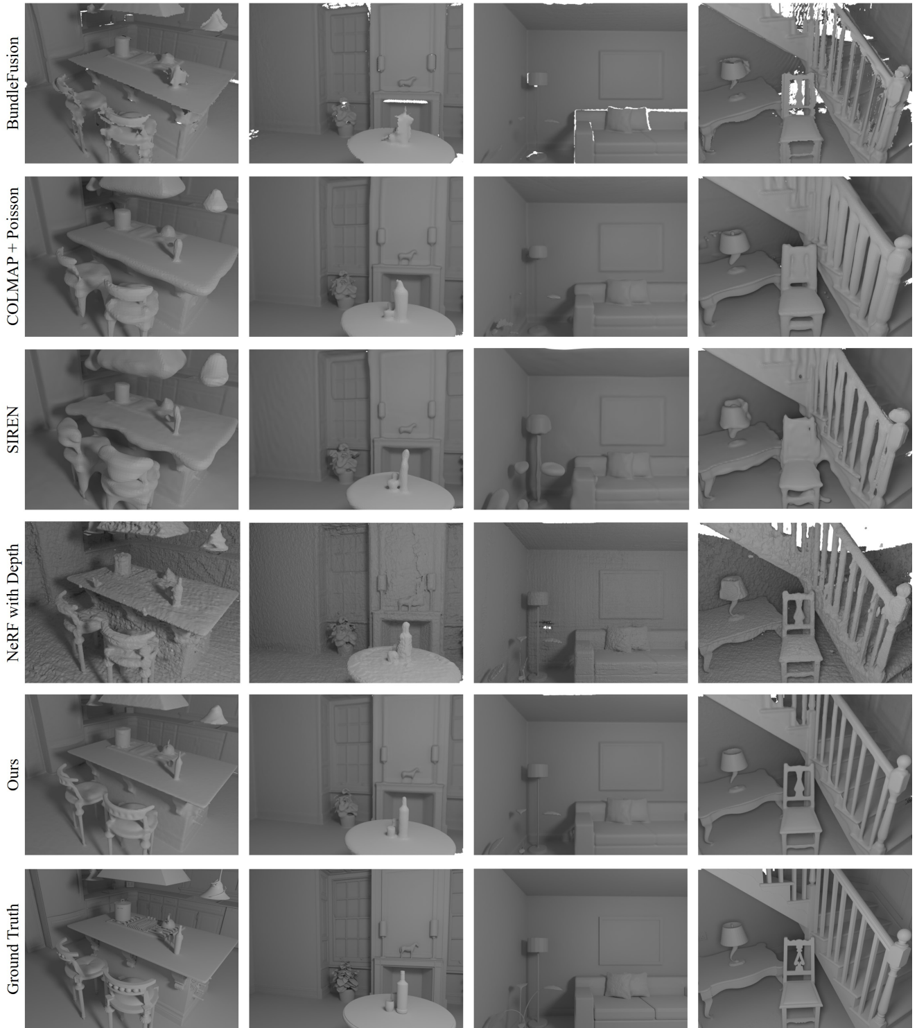
Figure 14. We show a qualitative comparison of synthetic scene reconstructions obtained using our method and several baseline methods. The BundleFusion reconstruction is incomplete in some regions, screened Poisson and SIREN attempt to fit noise in the depth data, while the NeRF reconstruction suffers from noise in the density field. Our method manages to fill in gaps in geometry, while maintaining the smoothness of classic fusion approaches.
