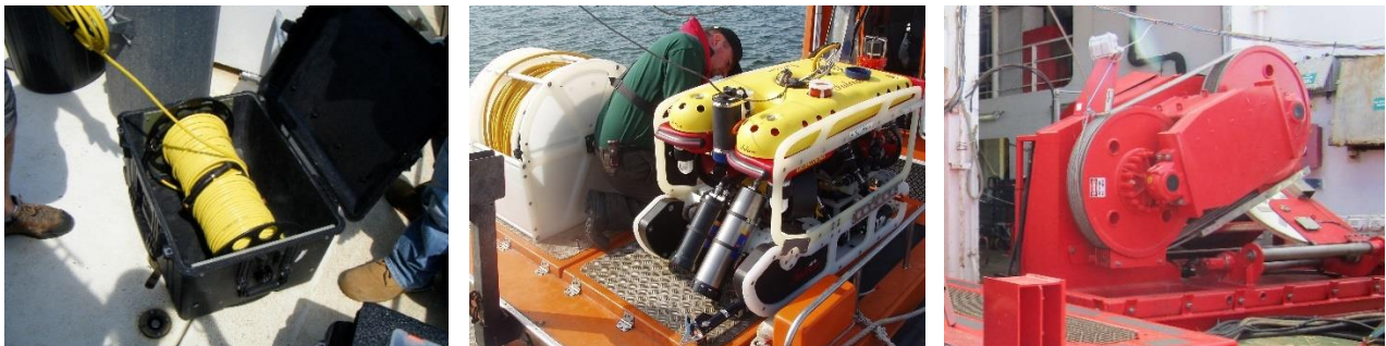
Figure 2. From Left-Right increase in length of tether and storage requirement for a Class 1 observation ROV (VideoRay) to a Class 2 observation ROV (Seaeeye Falcon) and to a work class ROV (Isis). (L-R images supplied by Marcus Shirley, Tim Mackie and Josh Davison).
