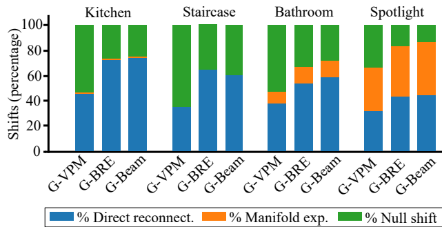
Fig. 12. Shift statistics after 30 minutes of rendering. For scenes dominated by specular and glossy transport (e.g., as in BATHROOM and SPOTLIGHT), shift mapping is more costly due to additional manifold exploration steps. Mixed shift reduces the need to perform manifold exploration by reusing photons for shift mapping, thus retaining the efficiency of gradient-domain methods.
