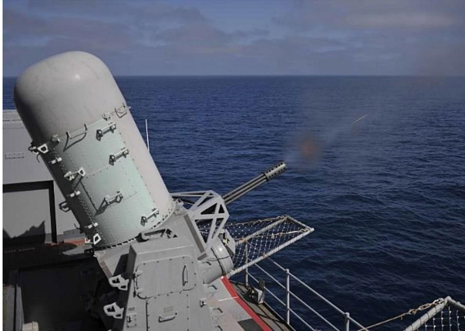
Figure 1. CIWS on the USS *Nimitz*. Source: U.S. Navy (2019).
