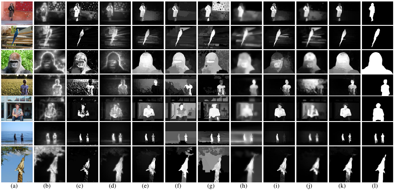
Fig. 12. Examples of saliency detection results: (a) Input image ; (b) CA; (c) GC; (d) PCA; (e) MR; (f) HS; (g) LMLC; (h) MS; (i) LPS; (j) MAP; (k) OURS ; (l) Ground truth . Our solution obtains the saliency maps close to the ground truth.
