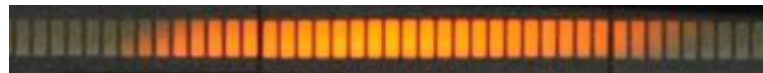
Figure 8: Influence of the opening time of a mechanical shutter on the image of an LED line. The LEDs in the middle are more exposed than the LEDs on the ends.
