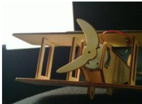
Figure 11: Close-up of the propeller as shot with the Nokia Lumia 1020 in smart mode using an electronic rolling shutter. The image of the propeller is deformed by the rolling shutter.
