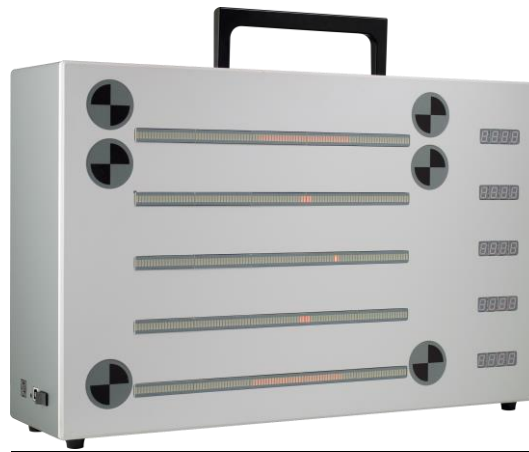
Figure 1: The DxO LED Universal Timer with five LED lines of 100 LEDs each. Six positional markers are used to automatically detect the timer in images; results are displayed on the right.
