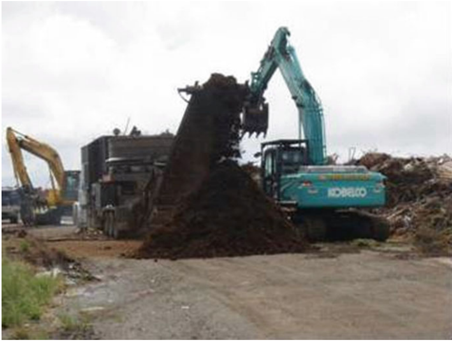
Fig. 4 Processing of urban, source separated, green waste to reduce volume for landfilling
