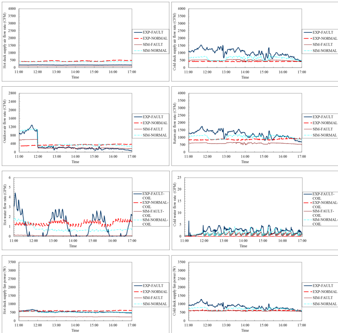
(b) Air &amp; water flow rates and supply fan power consumptions in dual duct system AHU
