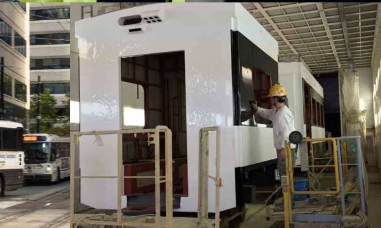
changes or service disruptions; Expanded section of a light rail vehicle on the assembly line; New Compressed Natural Gas Cruiser Bus; NJ TRANSIT's Music in Motion program entertains customers at several stations and terminals.
