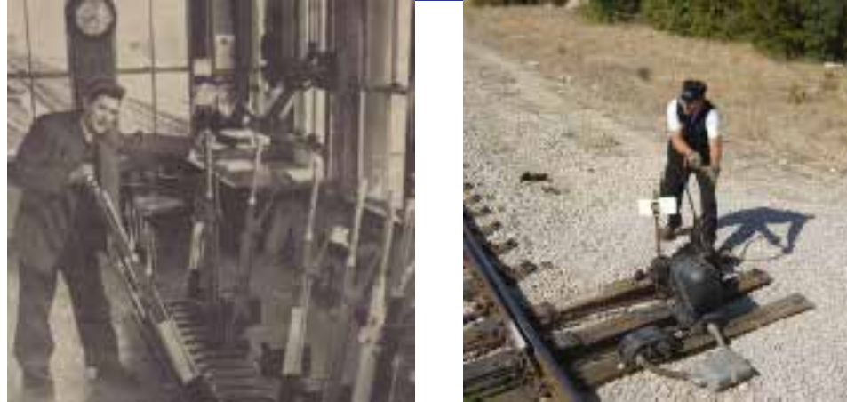
Manual switch throwing is still required at the Waldwick Yard to allow trains to turn back towards New York. This 100+ year old system is slow to operate and places conductors in harm's way.
