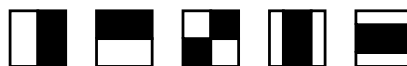
Figure 8: Haar features types used to generate one of the representations provided by the competition organizers.
