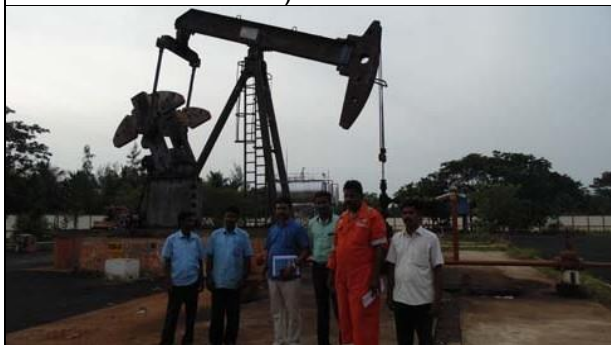
Sucken Rod Pump mechanized oil well near Koothanallur, Thiruvapur (Location: 10°44'08.67"N 79°29'44.71"E)
