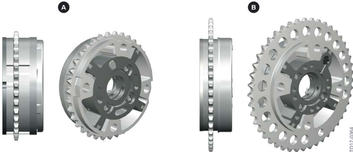
VANOS unit B46 engine and B46TU/B48TU engines
