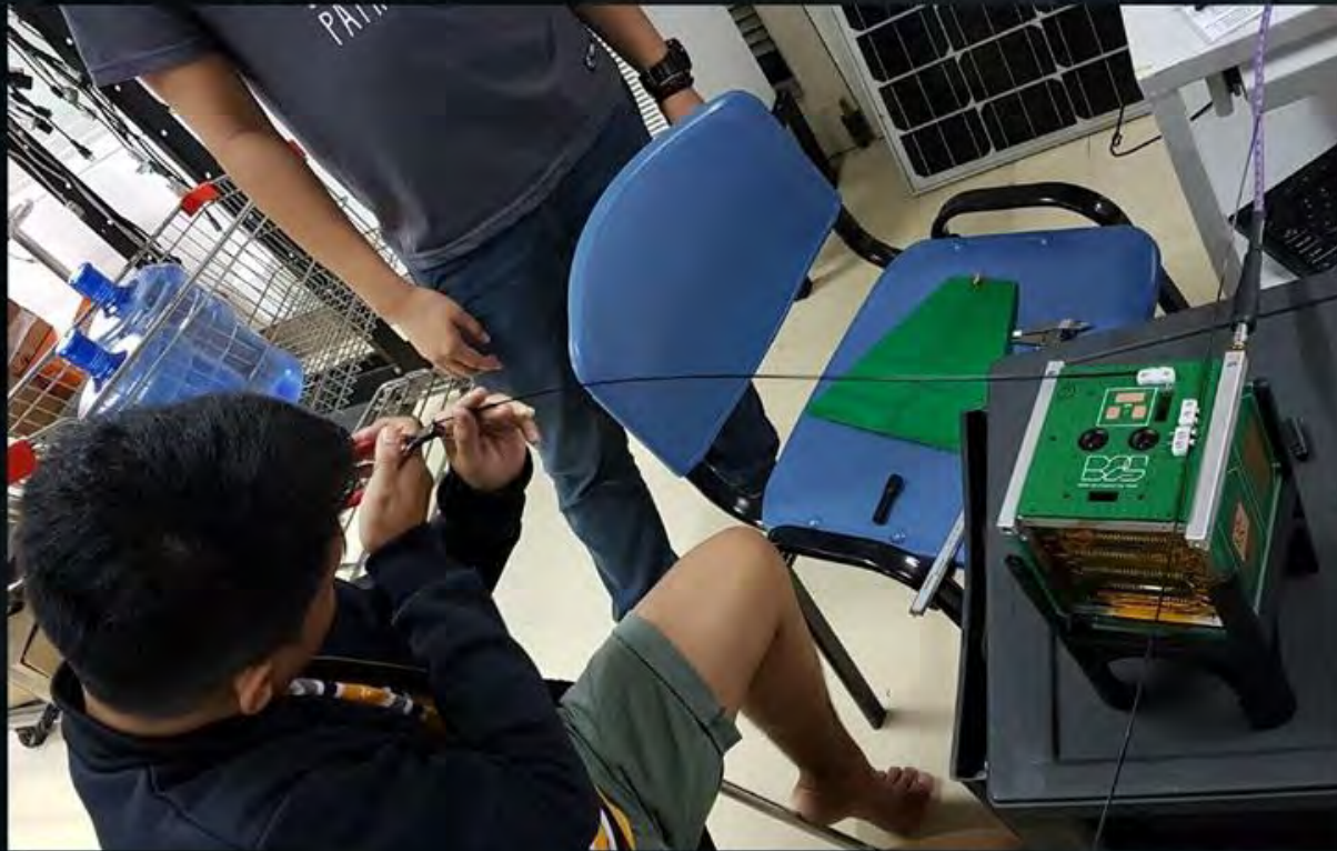
BIRDS 2S member Bryan Custodio cutting the antenna length
