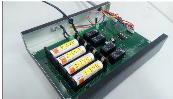
Battery charge-discharge hardware
