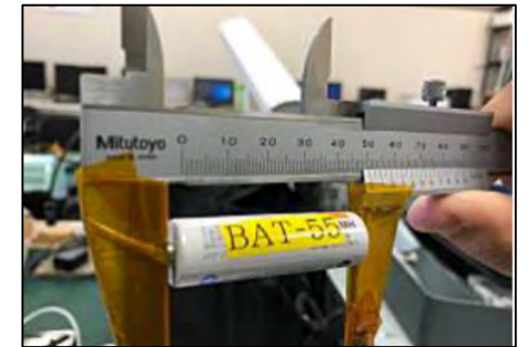
A scale and a caliper are used to measure battery weight and dimensions, respectively.
