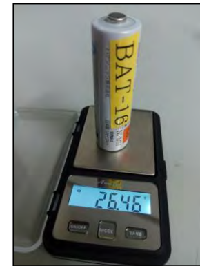
A scale and a caliper are used to measure battery weight and dimensions, respectively.
