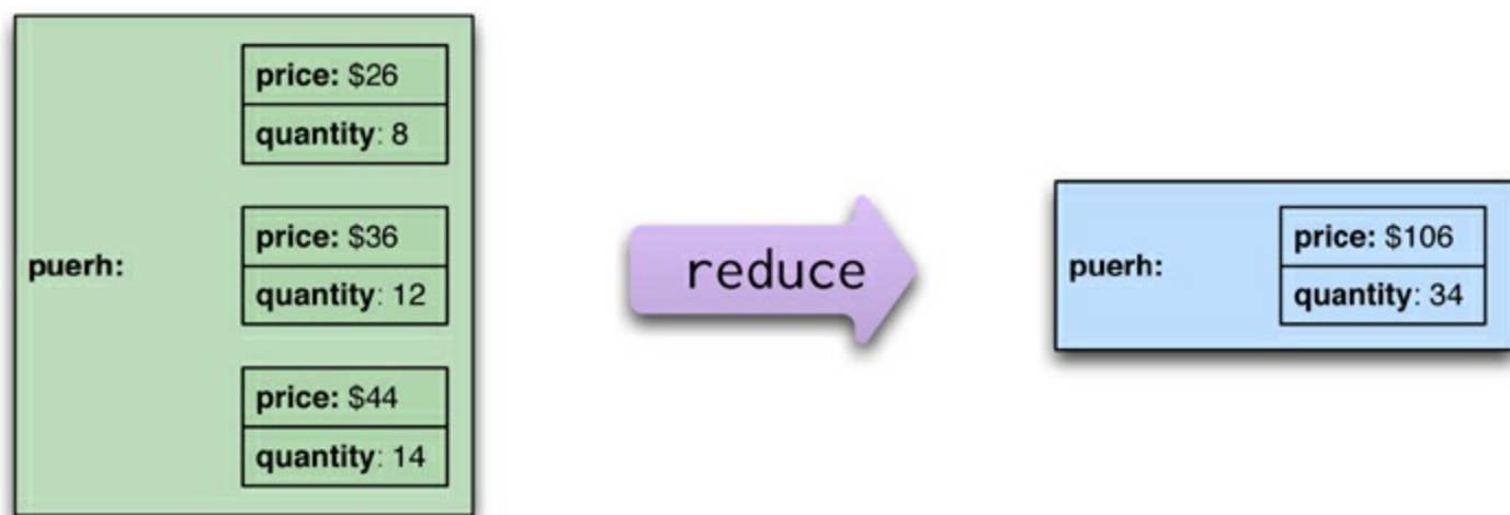
Figure 7.2. A reduce function takes several key-value pairs with the same key and aggregates them into one.
