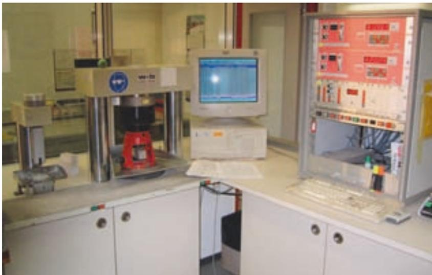
Fig. 37: core compression testing
