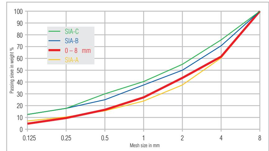
Fig. 25: dry sprayed concrete grading curve
