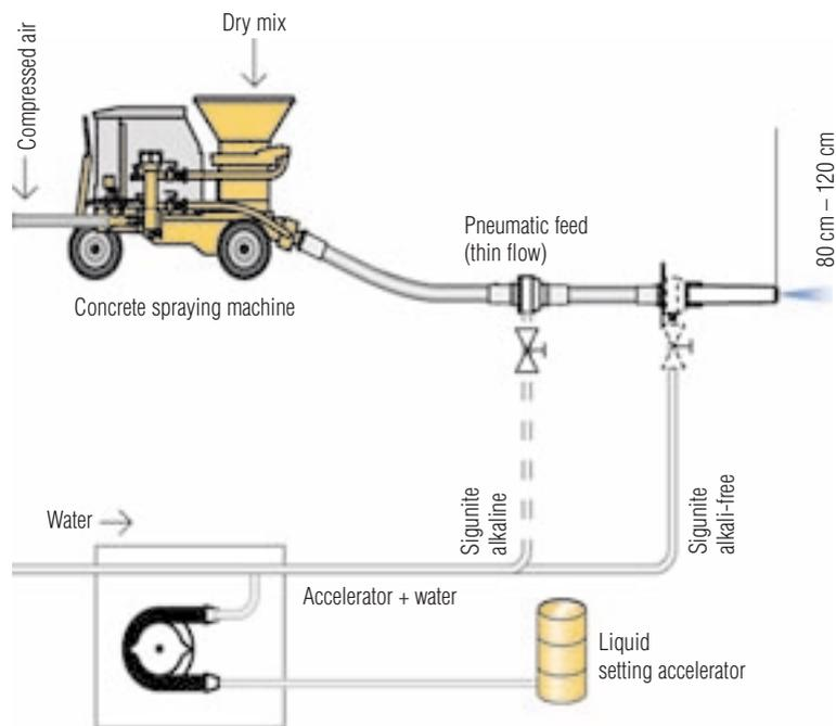
Fig. 51: thin-flow process for dry sprayed concrete
