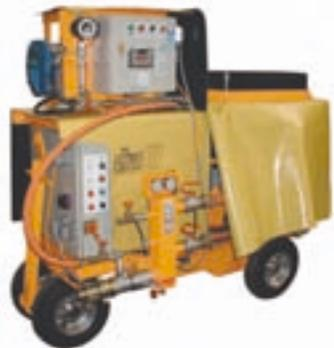
Fig. 53: Aliva®-263 Extended by metering unit
