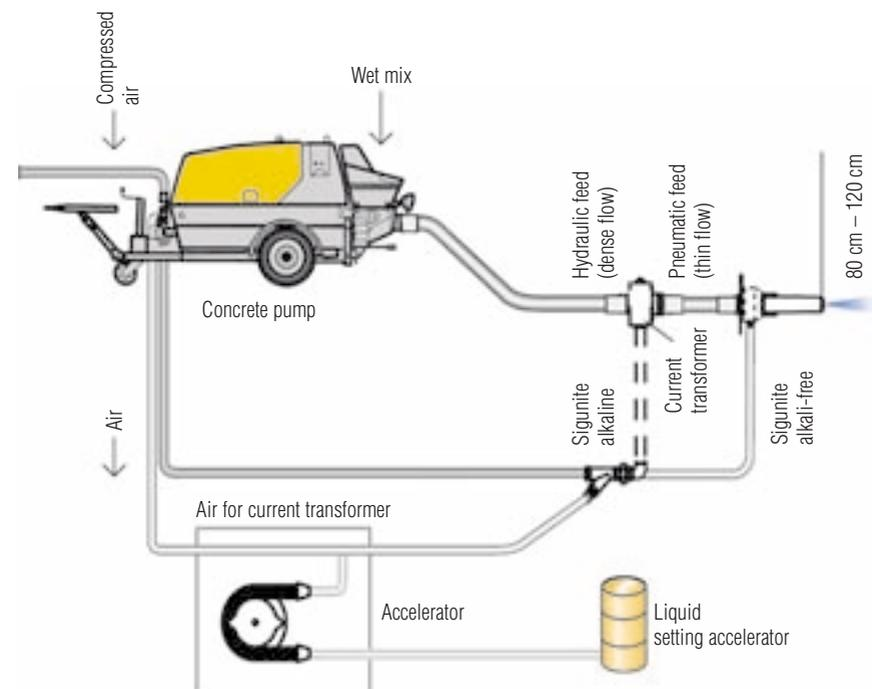
Fig. 39: dense-flow process for wet sprayed concrete
