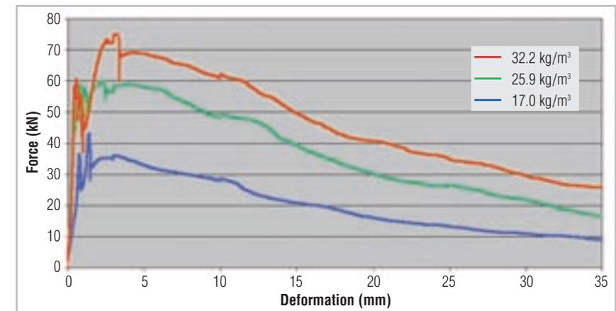
Fig. 20: plate test SIA 162/6, Steel fibre Dramix RC-65/35-BN
