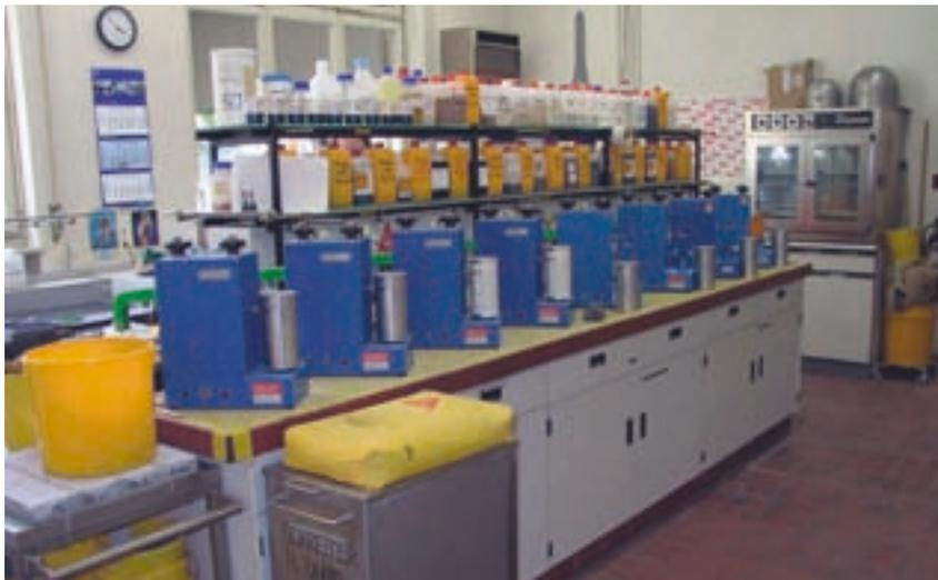
Fig. 14: Equipment for measuring the setting conditions
