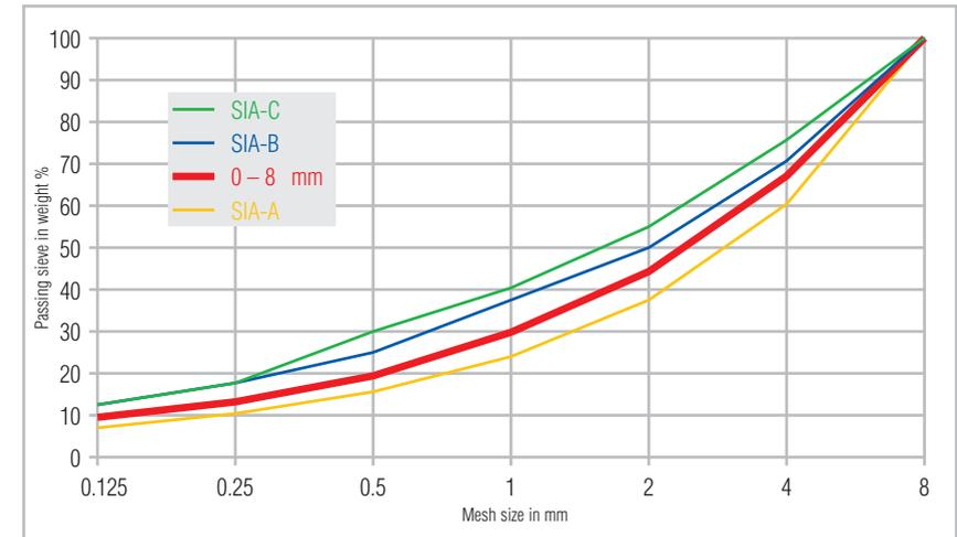
Fig. 23: grading curve of wet sprayed concrete, dense-flow process
