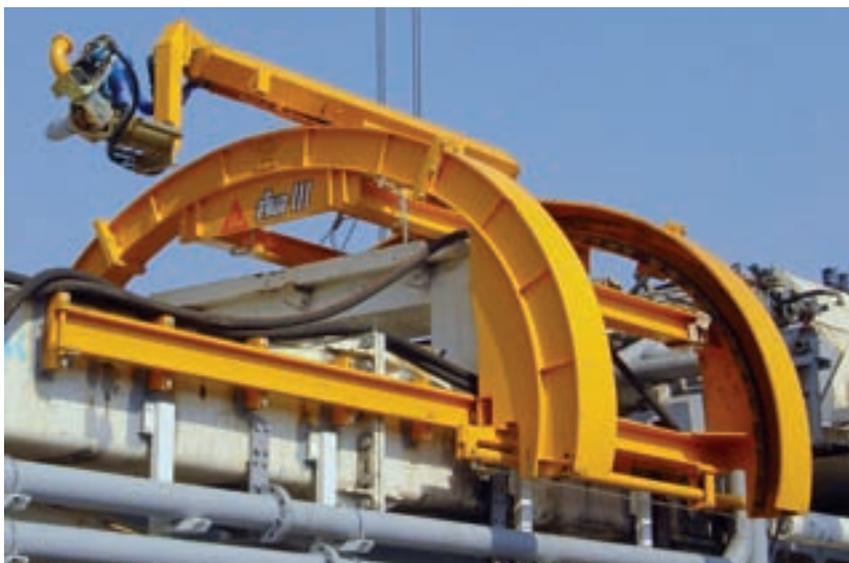
Fig. 11: TBM-spraying robot with telescoping spraying boom
