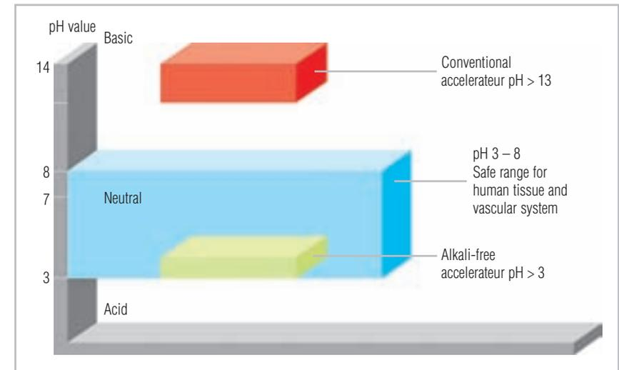
Fig. 13: List of setting accelerators
