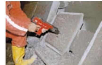
Fig. 36: very early strength from 1 to 15 N/mm<sup>2</sup> with bolt firing method
