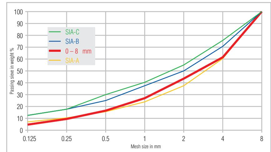
Fig. 24: grading curve of wet sprayed concrete, thin-flow process
