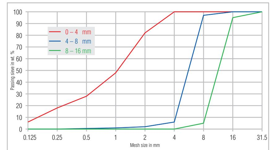
Fig. 12: Particle size distribution of individual components
