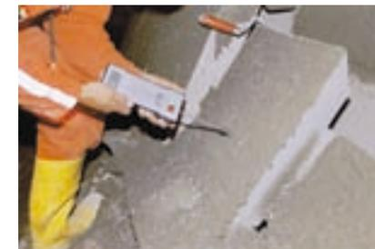
Fig. 35: very early strength from 0 to 1 N/mm<sup>2</sup> with needle penetration method
