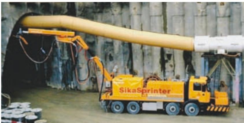
Fig. 4: Driving sprayed concrete laboratory
