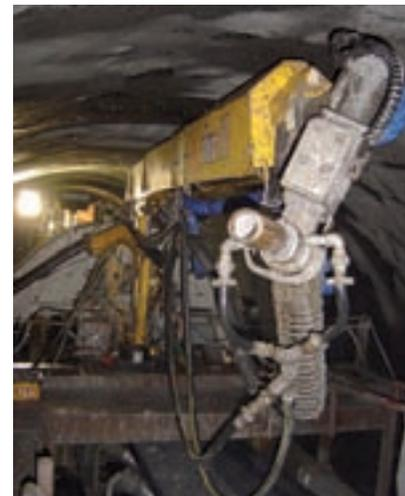
Fig. 47: Spraying robot with telescoping boom on the tunnel boring machine Karahnjúkar in Iceland
