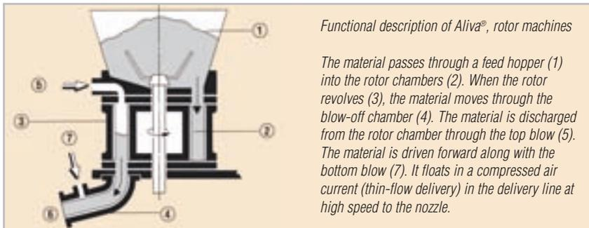
Fig. 52: schematic cross-section of Aliva® rotor machine
