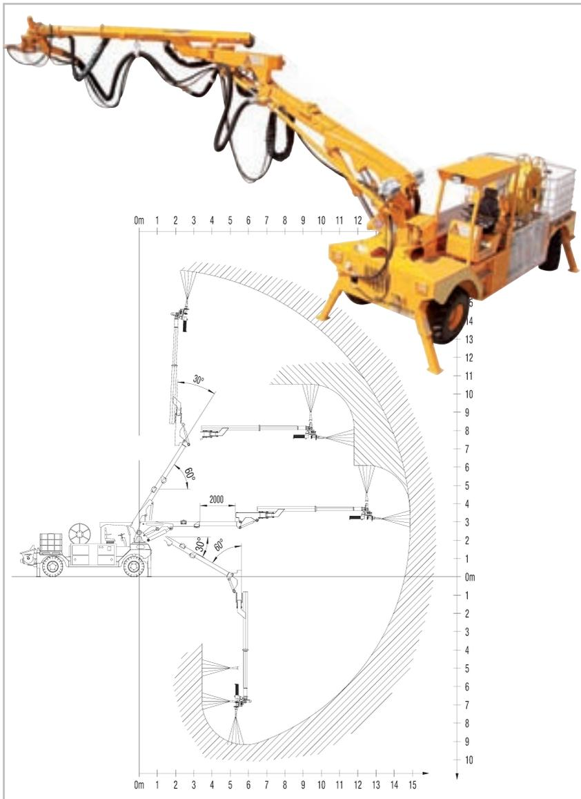
Fig. 45: Sika®-PM 500 with range diagram
