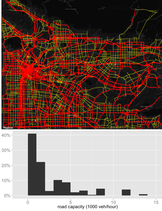
Fig. 1. The map of Los Angeles, CA used for the present study composed of 28,376 arcs and 14,617 nodes extracted from OpenStreetMap. Information for each edge includes the free-flow travel time, length, capacity, and speed limit. Links with capacity less than 1000 vehicles per hour are considered low-capacity (in yellow) while links with 1000 vehicles per hour or more are considered high-capacity (red). The histogram of the different road capacities are shown in the bottom figure, with more than 40% of low-capacity links.
