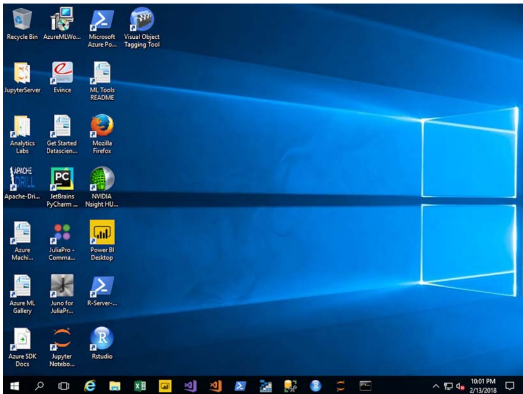
Figure 17.5 Data science virtual machines (DSVMs) are available for Windows and Linux. This Windows Server 2016 DSVM comes with several data science applications preinstalled, such as R Server, Jupyter Notebooks, and Azure Machine Learning Studio. DSVMs let you quickly get up and running with processing big data and building ML algorithms.
