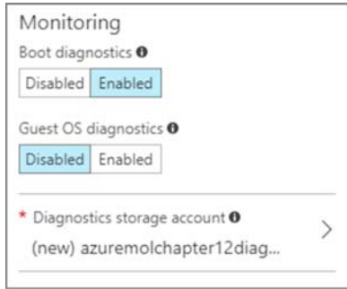
Figure 12.1 By default, boot diagnostics are enabled when you create a VM in the Azure portal. A storage account is created, which is where the boot diagnostics are stored. In a later exercise, you review and enable guest OS diagnostics, so don't enable them right now. For production use, I recommend that you enable both boot diagnostics and guest OS diagnostics for each VM you create.
