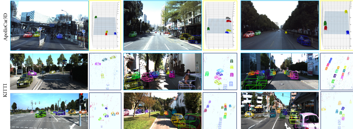
Figure 5. Qualitative examples under diverse scenarios. The top row are the results on the ApolloCar3D instances, and the bottom 2 rows show the results on some image frames of the KITTI tracking dataset. The system is capable of estimating the shape and pose (without scale-factor ambiguity) of objects. The images of the scenes contain the projection of the estimated shapes of cars.
