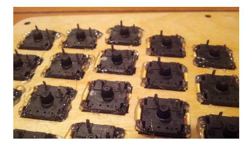
Melt a blob of solder onto each pin as you go before attaching anything else; this will make it much easier to hold the diodes and wires in place.
