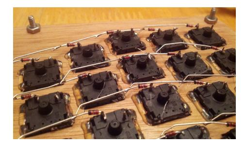
Once you've soldered a full row of diodes, you'll need to deal with the legs. Trim the remainder of the negative leg that extends below the switch contact, and solder the positive leg to the next diode in. Be sure to solder each positive leg to the next positive leg. The innermost column of diodes won't connect to anything yet, so you can trim their positive legs. They will get connected in the last step.
