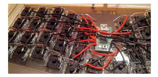
Next we'll connect the Teensy 2 microcontroller. All around the edge of the microcontroller board are "pins" (holes that don't actually have pins attached to them) which are labeled with a number and letter; we'll be wiring into pins D0-D3, B0-B7, and F4-F6, so locate these before starting. Note that pins D0-D3 and B0-B3 are consecutive on the Teensy, while higher pin numbers are scattered around the board.
