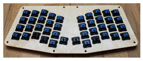
Start by placing your switches on the switch plate. The red stem (or black in some cases) switches should go where you intend to place the modifier keys. See the cheat sheet for a recommended positioning. Orient the switches so that the small notch on each one points to the bottom of the keyboard.
