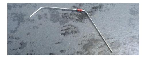
The positive leg of each diode needs to reach over the diode next to it to
