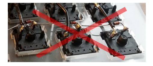
The above image shows incorrect diode usage; see how the positive leg of one is connected to the negative leg of the other, instead of positive to positive.
