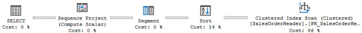
Figure 5-29: Execution plan to satisfy a Windowing function using a Segment and a Sequence operator.
